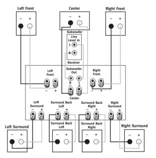
NOTE: If your receiver or amplifier has only one subwoofer output jack, then you will need to use a Y-connector (not included). Plug the male end of the Y-connector into your receiver or amplifier's subwoofer output jack, and connect each of the two female ends to separate RCA-type interconnects. Finally, plug the RCA-type interconnects into the line-level inputs on the subwoofer.
